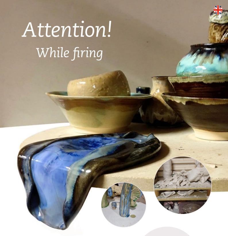
Never fire the clay higher than the recommended temperature. The flat, hanging product on the picture use to be a platter. It didn't only melt, it also got stuck to the kiln shelf.
